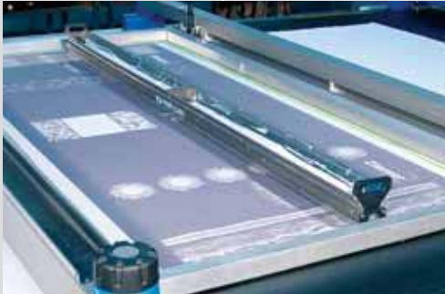
Magnetic steel squeegee. Mounted on the Magnet System with all advantages of the warp direction squeegee stroke, and for pressure-sensitive textile printing.
