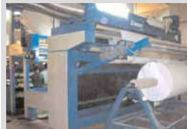
1 Optional pneumatic unbatching arm with digital drive system.
