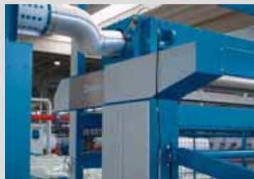
2 Cloth cleaning device with suction system, optionally available with brushing, blowing or beating system.
