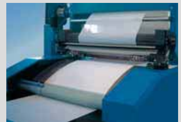
4 Cloth pressure roller with silicon rubber coating and servo drive with automatic speed adjustment for continuous oscillating roller movement.
