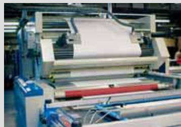
3 Individual cloth feeding systems available for any kind of woven, knits or special textile materials.
