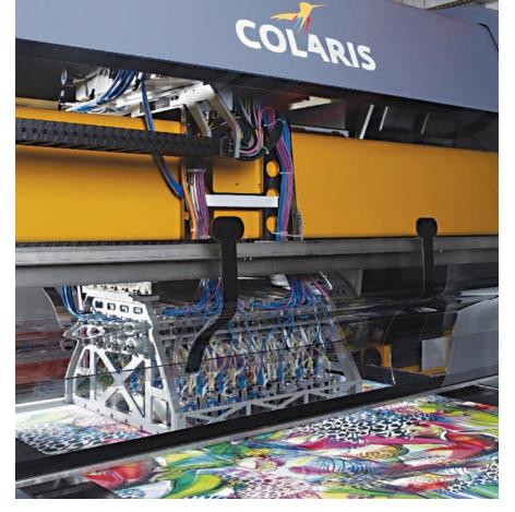
The Colaris series of printers from Zimmer Austria Inc. are compatible with a variety of colorants including reactive, disperse, acid, pigment and vat.
