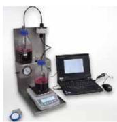
Ink Filtration Tester to check filterability of ink. The decrease of flow rate is measured over time to see how an ink performs during filtration.
