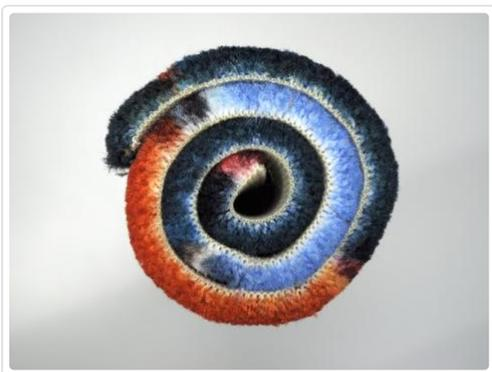
To achieve a fine appearance of the printed design, the carpet requires deep penetration of the inks (see the illustration above showing deep ink penetration). For this purpose, **ZIMMER AUSTRIA** has developed their own “Penetration Booster Technology”. This technology offers deep ink penetration under high printing speed for carpets from 200 up to 1,600 g/m<sup>2</sup>.
