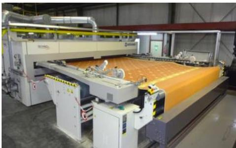
Stenter inlet to dryer
