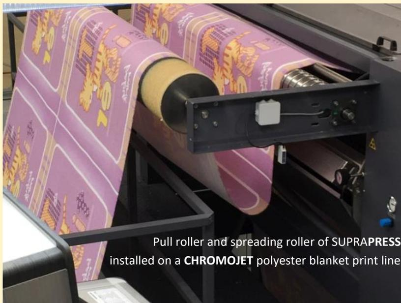
Pull roller and spreading roller of SUPRAPRESS installed on a **CHROMOJET** polyester blanket print line
