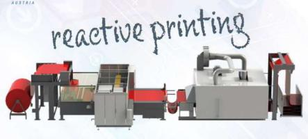
Reactive ink is used on fabrics made of cellulosic fibers such as cotton, linen, viscose, etc. It may also be used for printing on nylon substrates. For control of penetration and to achieve bright and brilliant colors the fabric needs a special inkjet preparation. Depending on the substrate, the preparation can be done as an inline or an offline process.
