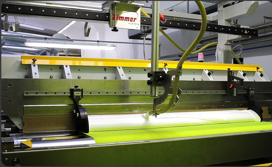
MAGNOROLL coating machine with MAGNOKNIFE
