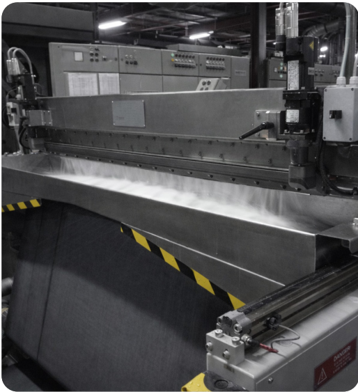
MAGNOJET with inline washing unit
