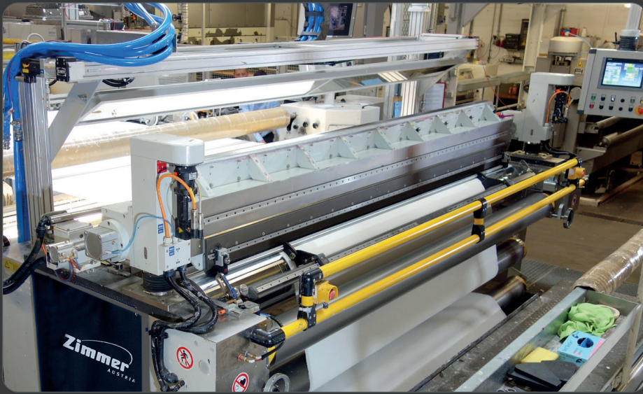
MAGNOROLL coating machine with MR 11 technology
