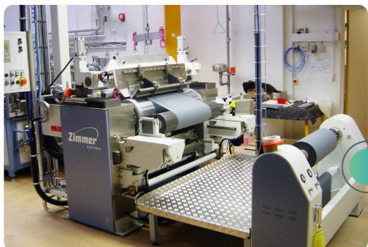
LABORATORY LINE KNIFE COATING
