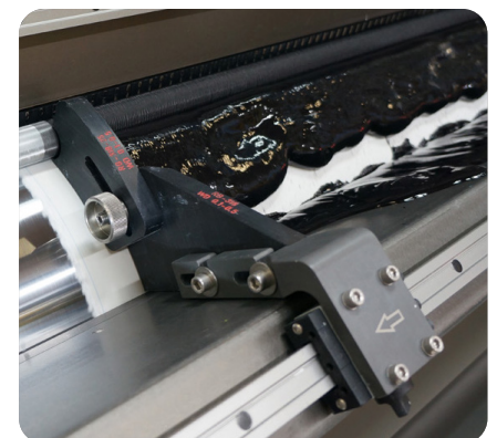
Paste reservoir with side limiters
