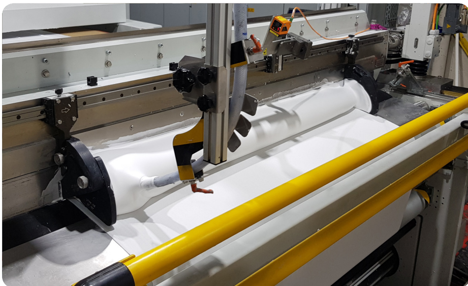
MAGNOROLL foam coating system with MAGNOKNIFE Over-Roll
