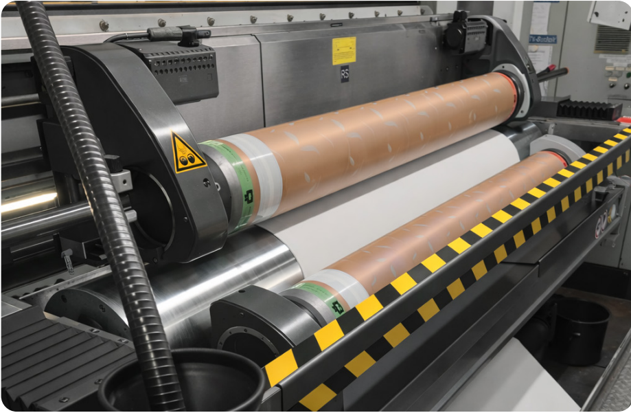
MAGNOROLL with two screen coating modules
