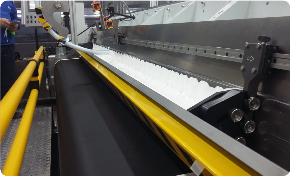
KNIFE coating with trough
