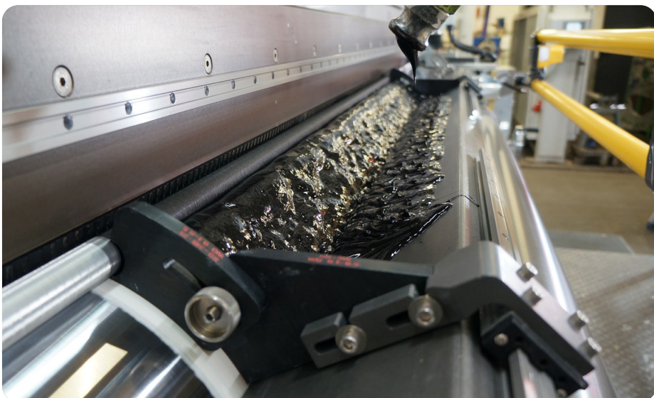
Magnetic Full-Surface Roll Coating MR 11
