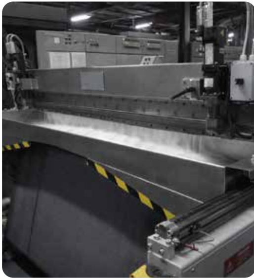
MAGNOJET with inline washing unit
