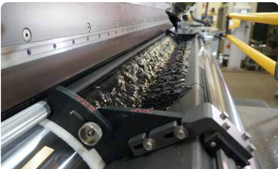
Magnetic Full-Surface Roll Coating MR 11
