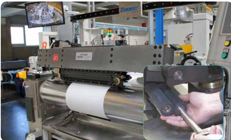
VARIOPRESS foam application with adjustable gear speed
