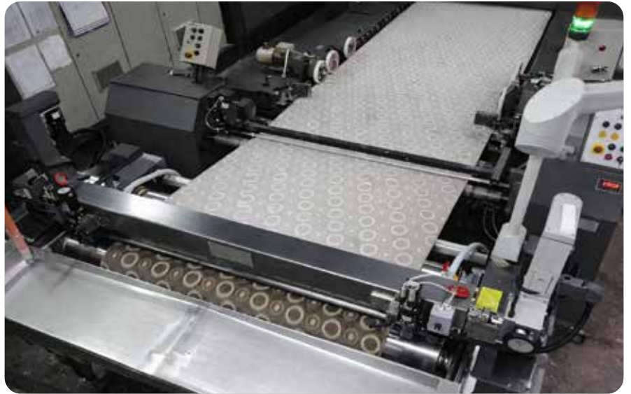
MAGNOJET foam coating unit installed in stenter frame line
