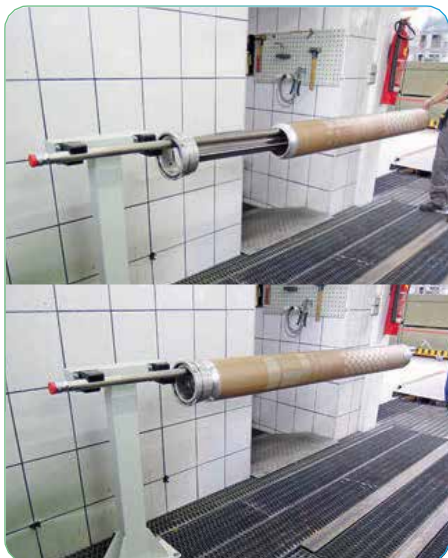
Pre-assembly of screen and squeegee
