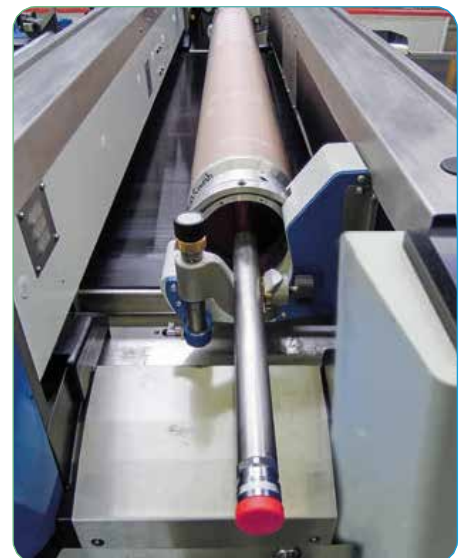
ROTASCREEN TU open bearing system
