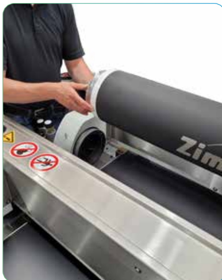
ROTASCREEN TG - screen set-up
