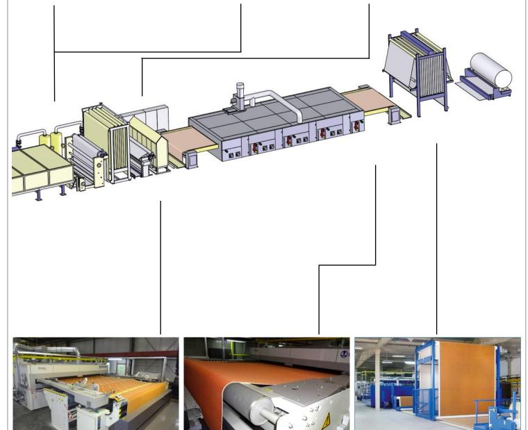
Stenter inlet to dryer
