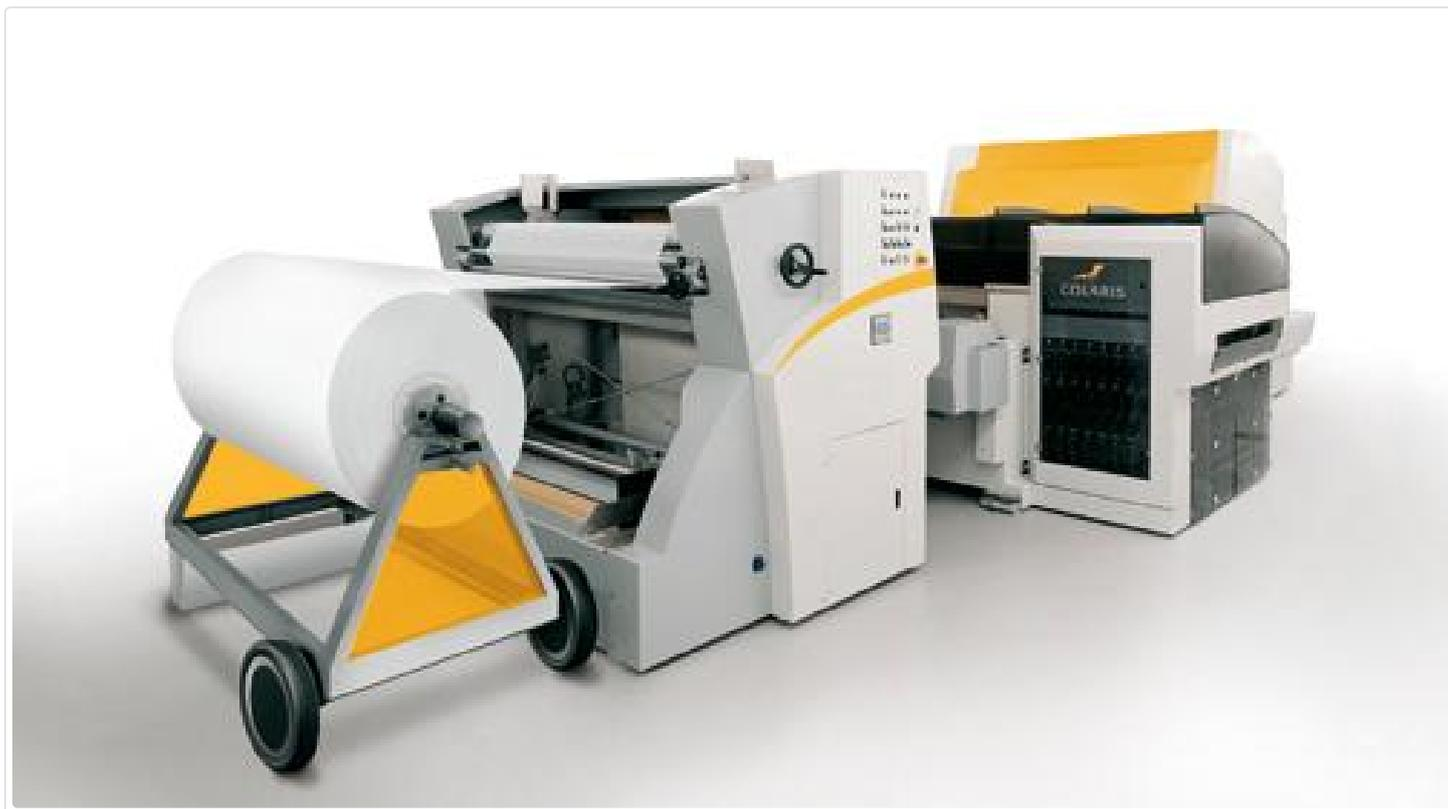
Zimmer offers the complete **COLARIS** technology along with the know-how used for operation. Production capacity up to 480 m<sup>2</sup>/h for the printing width of 180 cm; (per hour 260 linear meters)
